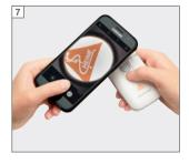
With the phone now in its case, the magnet on the connector keeps the phone in position on the focusing ring of the dermatoscope.
